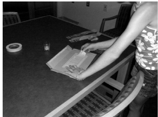
A two-inch wide strip has been cut from the center of the still-damp filter. Here it is placed on the glue-covered slides that have been taped to a new piece of cardboard.
